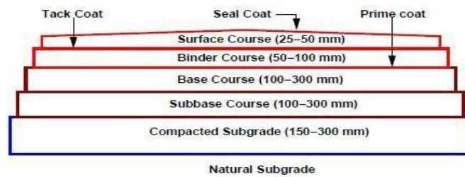
Typical cross section of a flexible pavement
